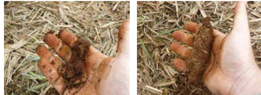
Figure 1 Forming a bolus (soil ball) in the field to determine soil stickiness.
